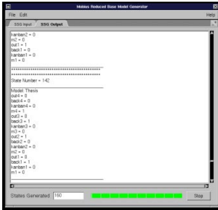
Figure 6: State-Space Generator Output
